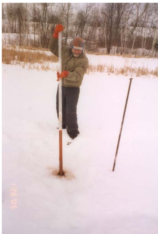
Photo 17 (bottom left). Tiller drawing up yellow boy sediment sample from Dober mine settling pond #1, 26 January 2005
