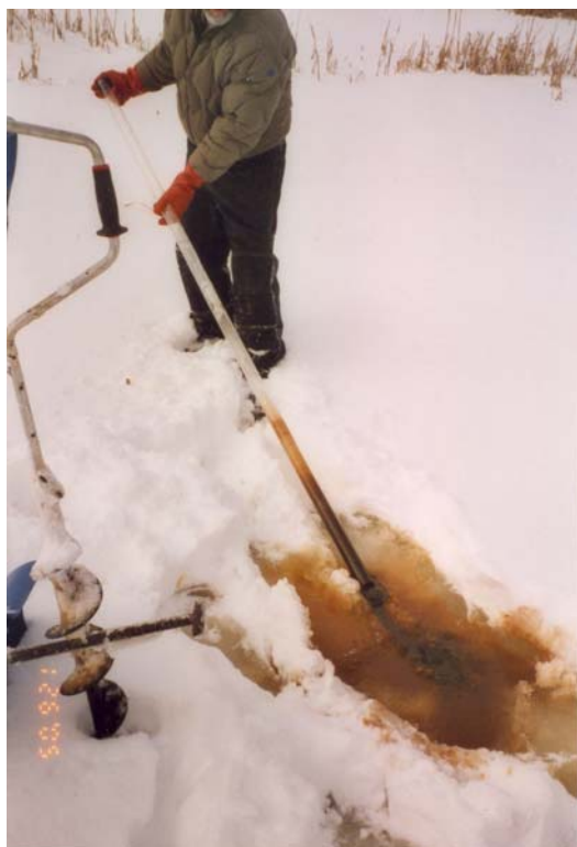
Photo 15 (top left). Tiller with bottom sample of Dober mine settling pond #1, 26 January 2005
