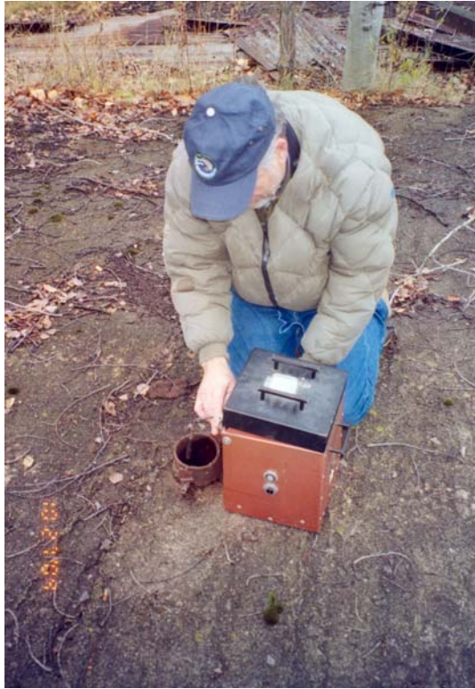
Photo 1 (top left). Tiller taking water level reading at Hiawatha #1 pipe shaft, 22 October 2004
