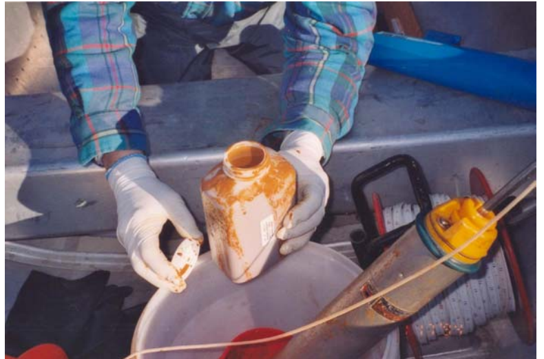
Photo 13 (middle right). Tiller with yellow boy sample taken from 75 foot depth in Dober mine pit, 23 November 2004
