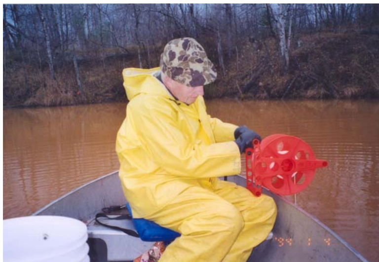
Photo 11 (bottom left). Johnson with Kemmerer rig on Dober mine pond, 10 November 2004
