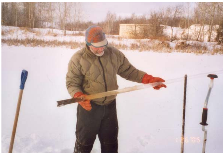
Photo 17 (bottom left). Tiller drawing up yellow boy sediment sample from Dober mine settling pond #1, 26 January 2005
